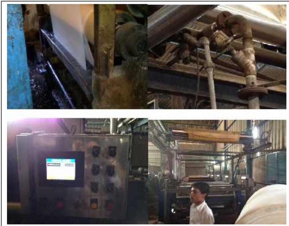
**Pilot measure:** Installed two separate water lines for jigger machines, for water filling (1.5 inch) with auto timer based controller to fill required quantity of water into jigger, for overflow (0.5 inch) line with auto timer controller which allows only 400 litre per 20 minutes and stops the water flow after one turn. Also the water supplied to the jigger is from condenser cooling water of caustic recovery
