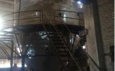
The spray dryer is a device mainly used in wall and floor tiles manufacturing industries as far as ceramic sector is concerned. Its main application is in formation of required size granules from the wet slip. Care must be taken that the density of the slip fed to the spray dryer must always remain the same to obtain the same size of granules, as varying density of feed forms granules of varying sizes.
