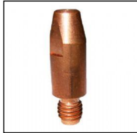
Figure 1: Before Cleaner Production: Copper welding nozzle
